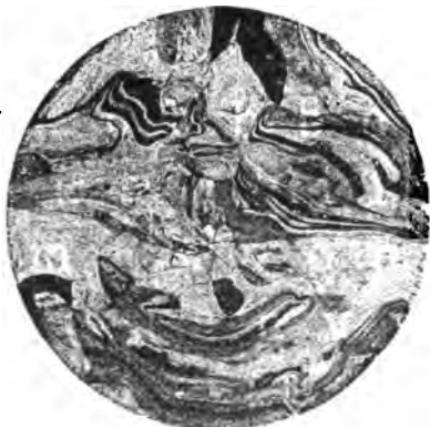
FIG. 56.—LOCOMOTIVE AXLE— "SPECIAL" IRON.
